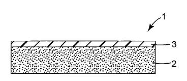
(57) Abstract: A single-coated adhesive tape without a backing substrate is provided. The single-coated adhesive tape comprises an adhesive layer having a thickness of 30 to 1000 um, which contains 50 to 95% by weight of a hot melt adhesive and 5 to 50% by weight of a film-forming component, and a non-tacky coating layer having a thickness of 0.01 to 15 µm is provided on one surface of said adhesive layer.
