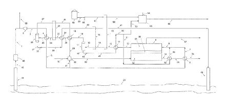
(57) Abstract: A method to extract methane from a coal bed seam with carbon dioxide produced and recovered from a fuel cell anode exhaust stream while simultaneously sequestering the carbon dioxide on the coal. The process produces methane to supply a fuel cell to generate electricity while reducing or eliminating GHG emissions.
