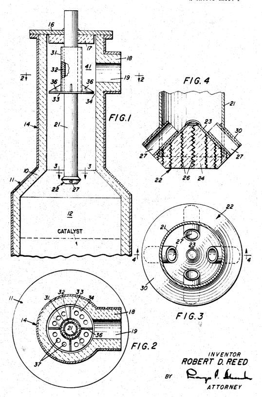
BURNER AND APPARATUS FOR REFORMING HYDROCARBONS
