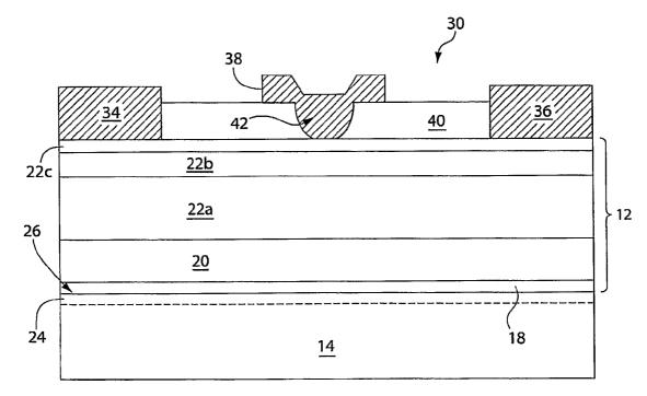
(57) Abstract: III-nitride material structures including silicon substrates, as well as methods associated with the same, are described. Parasitic losses in the structures may be significantly reduced which is reflected in performance improvements. Devices (such as RF devices) formed of structures of the invention may have higher output power, power gain and efficiency, amongst other advantages.
