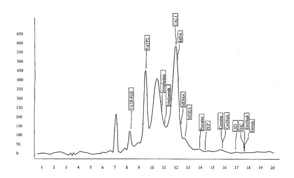
(57) **Abstract:** A method of detecting the presence of an analyte in an ion mobility spectrometer using an amide ionization reagent is provided. This method is particularly useful for the detection of peroxide-based explosives.
