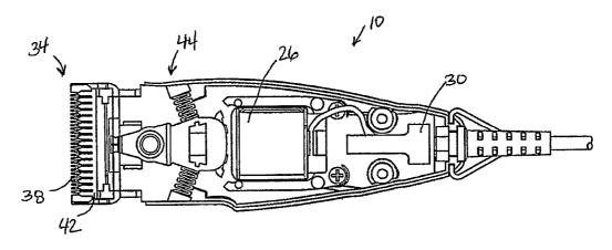
(57) Abstract: A hair clipper or trimmer (10) having an inner cavity (22) including a controller (30) and a pivot motor (26) operable to control a reciprocating blade at a speed greater than 3,600 blade strokes per minute. The hair clipper (10) or trimmer can also use a vibrato magnetic motor (26) operable to control a reciprocating blade at a speed greater than 7,200 blade strokes per minute.
