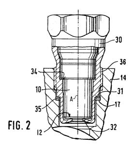
Drawings, illustrating preferred examples, wherein: FIG. 1 is a fragmentary axial view, partly in section, of a fuel injection plug with a heat protecting sleeve; and
