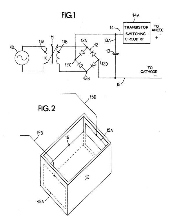
METHOD FOR REDUCING OR ELIMINATING MICROORGANISMS IN SUBSTANCES BY **ELECTRIC STIMULATION**
