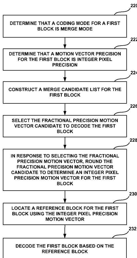
(57) **Abstract:** A device for decoding video data includes a memory configured to store video data and a video decoder comprising one or more processors configured to adaptively select motion vector precision for motion vectors used to encode blocks of video data.
