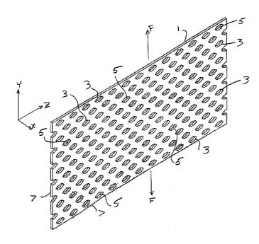
(57) Abstract: An implant member has a body made from biocompatible material, and this body has slits formed therein. The slits open when the body is subjected to tension. The implant member is made by providing a body member and forming slits in the body. The slits are dimensioned and disposed so that the slits open when force is applied to the body.
