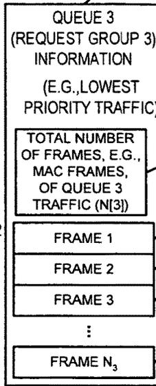
WT A MAPPING OF UPLINK DATA STREAM TRAFFIC FLOW FRAMES TO ITS REQUEST QUEUES
