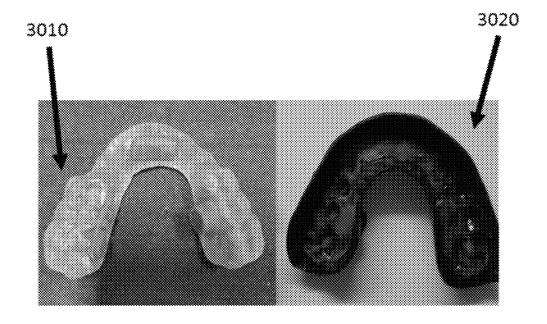
Figure 3: Sample 1 with the rigid 3D printed layer and electronics geometries (3010) and the completed sample with trimmed EVA (3020).
