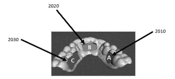
Figure 2: Three electronics geometries including the battery (A), the main circuit board (B), and the power circuit board (C).
