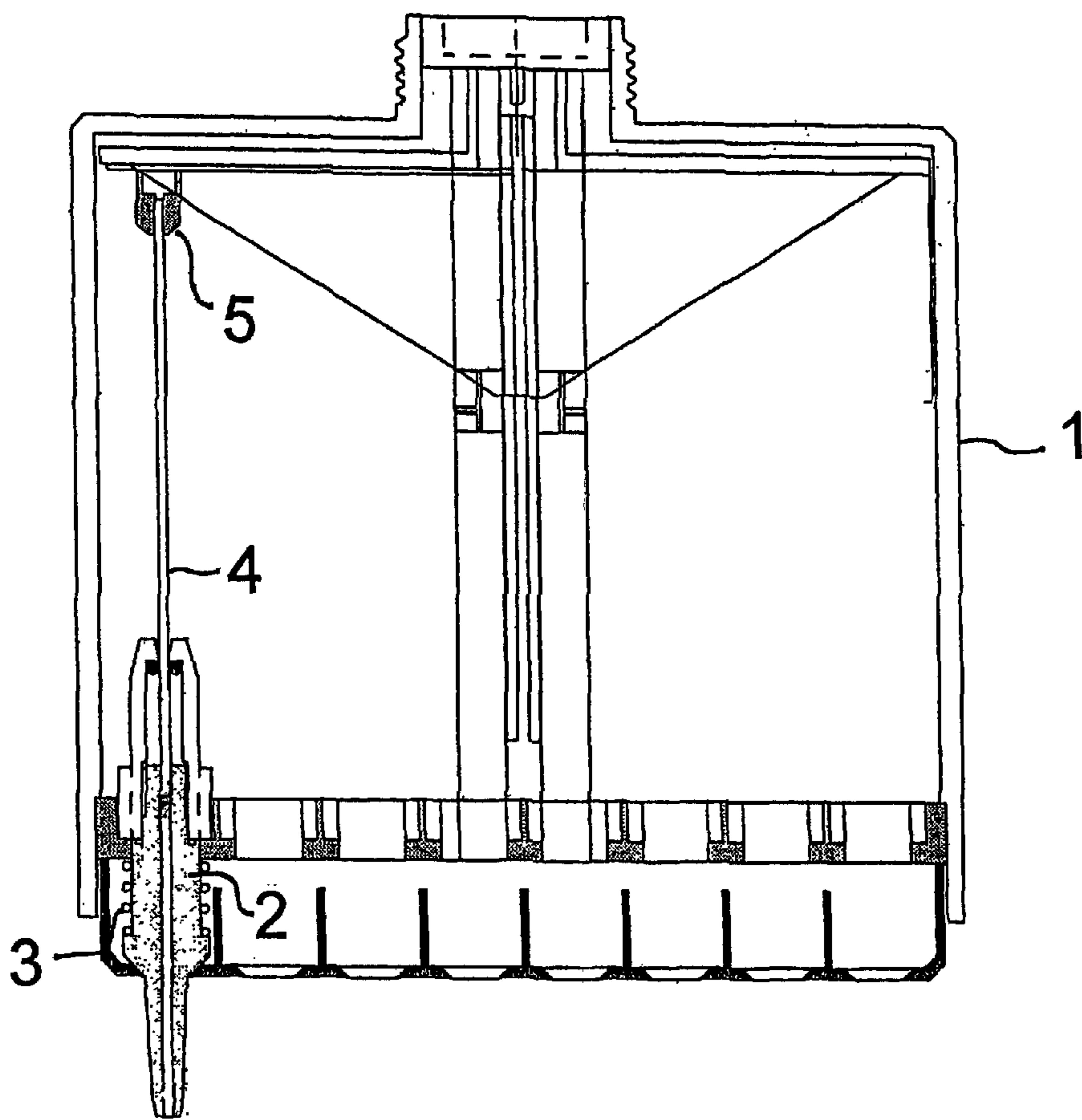
(57) Abstract: A multichannel pipette, the suction tube arrangement of which is arranged to be resilient, so that a disposable tip is attached similarly to each suction tube regardless of the shape and elastic characteristics of a tip rack. The pipette comprises a body and a plunger-cylinder system with suction tubes for each channel. Each suction tube is thus adapted to the body, that the suction tube is movable between two extreme positions in its vertical direction with respect to the body.
