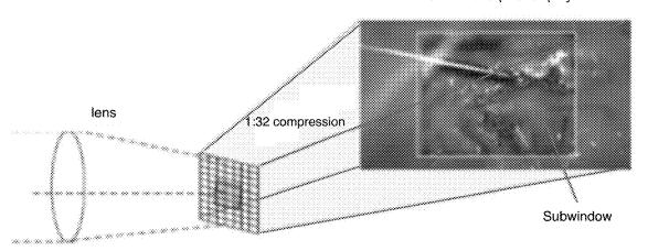
high resolution focal plane array 61440 x 34560 pixels
