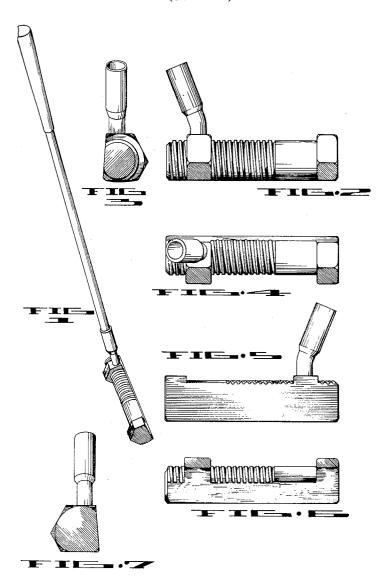
FIG. 1 is a perspective view of the putter, showing my new design,
