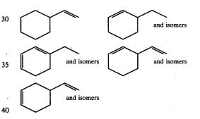
In the manner previously described, the ethylbenzene and vinylcyclohexene components of the product mixture can be converted to styrene in a second step dehydrogenation reaction in the presence of molecular oxygen (or nitrobenzene) and a Group VIII metal catalyst.
