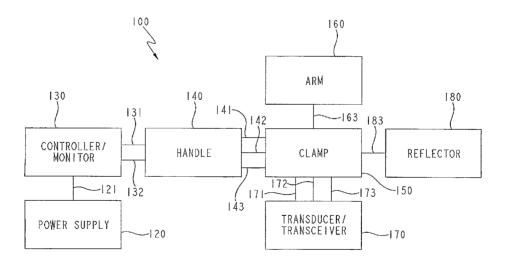
(57) Abstract: A surgical clamp is provided, including a first arm, a second arm, a source of high intensity non-focused ultrasound, and a reflector. An organ or biological tissue, or portion thereof, may be received by the clamp.
