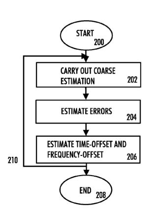
(57) Abstract: The invention is related to a synchronization method in a communication system. The invention includes: carrying out a coarse time offset and frequency offset estimation, first estimating errors in the coarse time-offset and frequency offset estimation by using a maximum-likelihood time-offset estimation and joint optimisation of time-offset and frequency-offset, second estimating frequency offset and time offset by using error estimates in a closed tracking loop.
