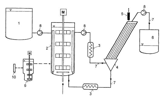
(57) Abstract: The present invention relates to a continuous process for high cell density cultivation of suspended animal or plant cell lines with the aim of efficiently producing biological products. The invention also relates to units and apparatuses in which the process according to the invention for cultivating suspended animal or plant cell lines can be carried out.
