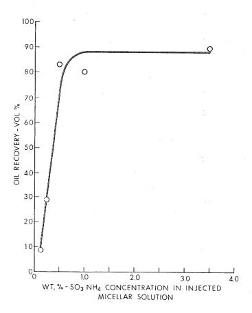
OIL RECOVERY VS - SO3 NH4 CONCENTRATION MICELLAR SOLUTION
