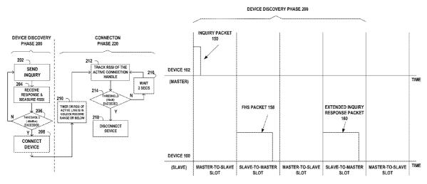
TIMING DURING A DEVICE DISCOVERY PROCESS, FOR EXAMPLE A BLUETOOTH INQUIRY PROCESS
