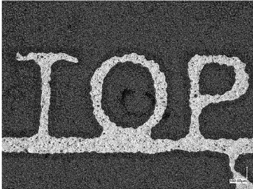
REFLECTION CAPTURE EXAMPLE WITH OPTICAL MICROSCOPE (150X) OF TRANSFER FOIL WITH ETCHED REFLECTIVE LAYER
