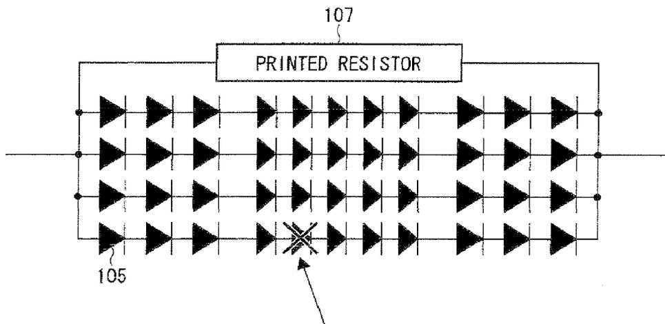
If one LED chip is open-defective in a row, for example, the other 10 LED chips in the row do not emit light.
