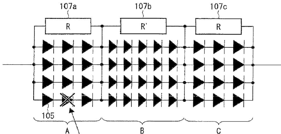
If one LED chip in a group in a row is open-defective, for example, the other 2 LED chips in the same group in the row do not emit light. However, remaining 8 LED chips in the other groups in the row still emit light.
