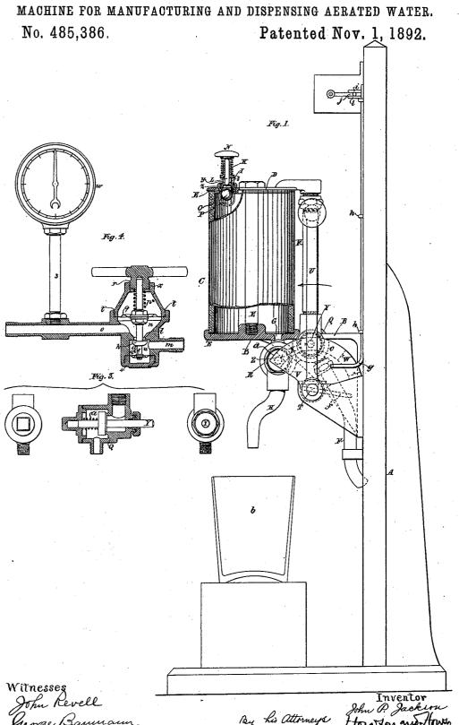
MACHINE FOR MANUFACTURING AND DISPENSING AERATED WATER.
