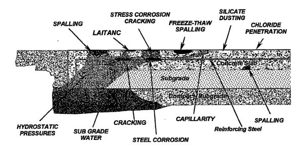
Figure 2. Common water associated problems in concrete pavements.
