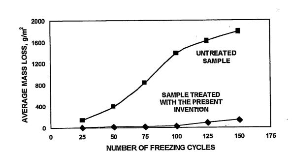
Figure 4. Results of freeze and thaw test for a concrete sample treated with the present invention compared to an untreated sample.
