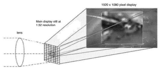
high resolution focal plane array 61440 x 34560 pixels
