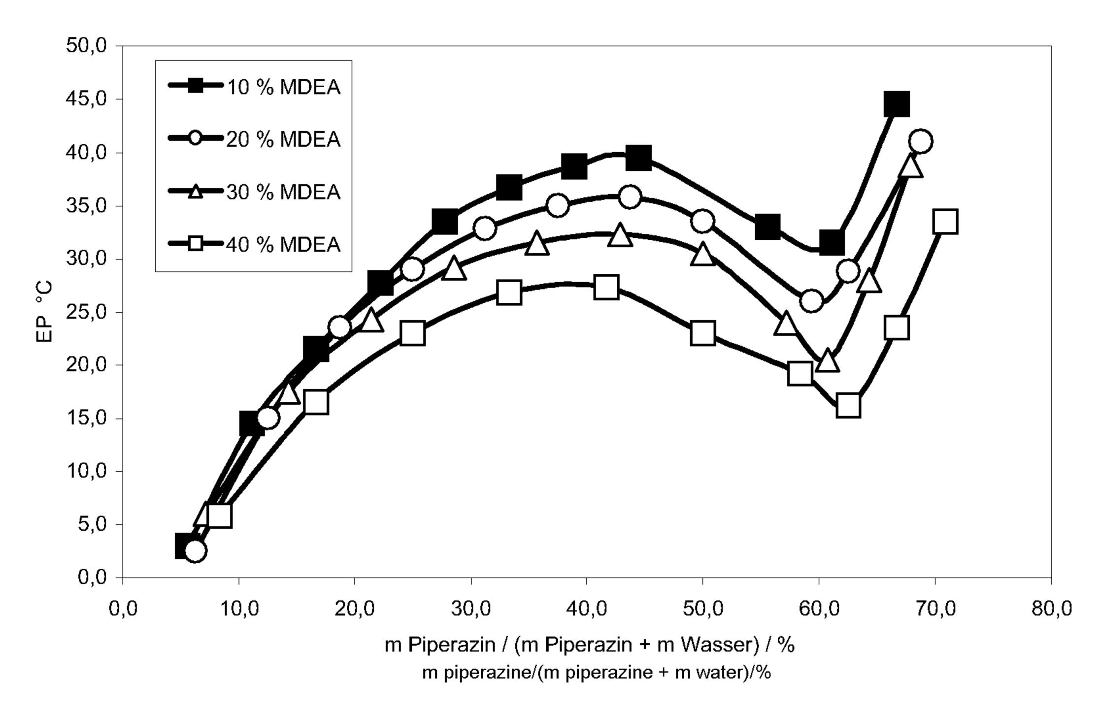
(57) Abstract: A premixture for preparing an absorbent for removing acidic gases from fluid streams is described. The premixture comprises at least one alkanolamine, piperazine and water, the premixture having a total amine content of more than 65% by weight and the molar ratio of water to piperazine in the premixture being from 1.6 to 4.8. The premixture is characterized by a low solidification point. It is diluted with water and/or alkanolamine to give the ready-to-use absorbent.
