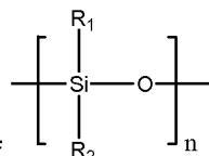
[0017] A “polysiloxane” refers to a moiety of  $\left[ \begin{array}{c} R_1 \\ | \\ -\text{Si}-\text{O}- \\ | \\ R_2 \end{array} \right]_n$  in which  $R_1$  and  $R_2$  are independently a monovalent  $C_1-C_{10}$  alkyl,  $C_1-C_{10}$  ether,  $C_1-C_{10}$  fluoroalkyl,  $C_1-C_{10}$  fluoroether, or  $C_6-C_{18}$  aryl radical, which may comprise hydroxy group, primary, secondary, or tertiary amine group, carboxy group, or carboxylic acid;  $n$  is an integer of 4 or higher.
