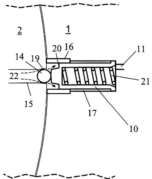
**VCT MECHANISM HAVING A LOCK PIN
