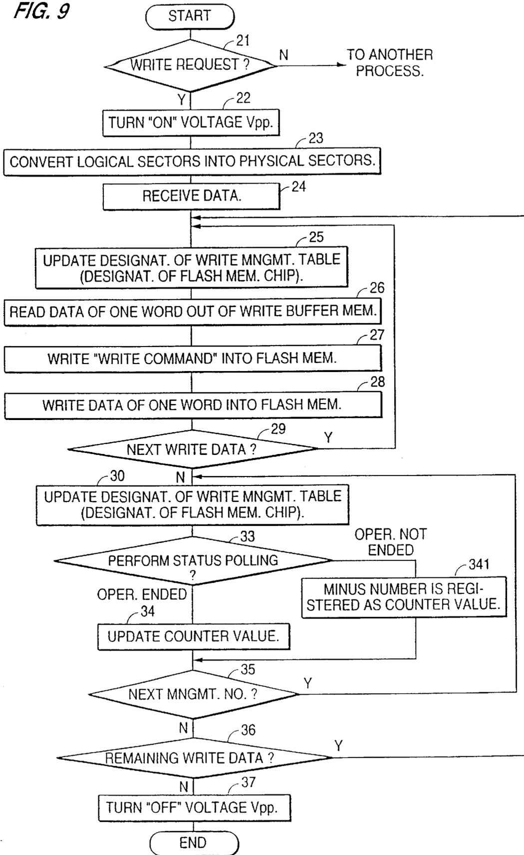
**SEMICONDUCTOR STORAGE DEVICE IN WHICH COMMANDS ARE SEQUENTIALLY FED TO A PLURALITY OF FLASH MEMORIES TO CONTINUOUSLY WRITE DATA**
