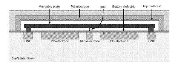
the one or more electrodes that cause the plate to move is reduced and capacitance modulation is reduced or even eliminated.
