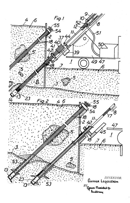
METHOD AND EQUIPMENT FOR MAKING TENSION ANCHORS
