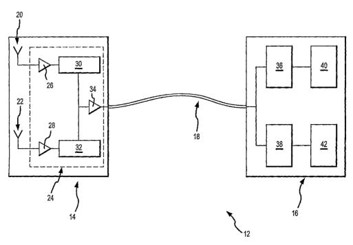
GPS signals. The two antennas may or may not be on a common ceramic substrate. Either of the two antennas may be a ceramic patch antenna or a helical antenna. The respective signals from each of the antenna as is amplified by a low noise amplifier, filtered, and then combined onto a single conductor and amplified prior to being provided on a single conductor routed through the vehicle to a remotely-located pair of receivers.
