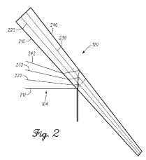
(57) Abstract: A wavelength combining apparatus (100) includes first and second optical devices. The first optical device (110) collects and collimates or focuses light from multiple laser light sources. The second optical device (120) includes multiple non-parallel dichroic surfaces to combine light received from the first optical device.
