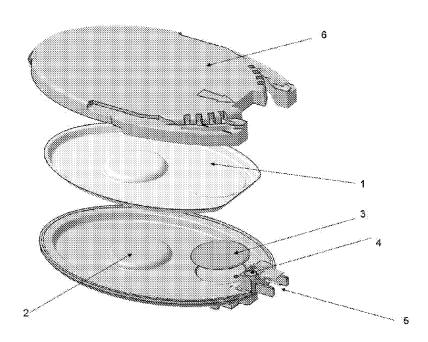
(57) Abstract: A polymeric container for storing a drug such as insulin which comprises a hard shell (2) and a flexible film (1), wherein both elements are made from the same material.
