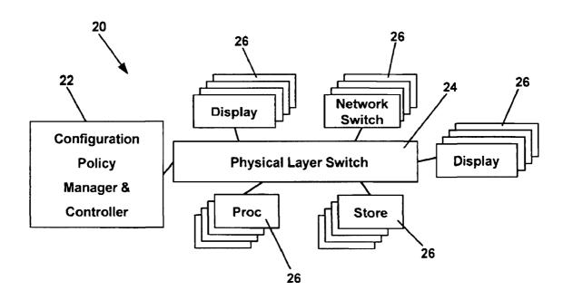
Proc Display Network Switch Store Guard Proc Display Store Network Switch Guard Store Network Switch FIG. 1 (Prior Art) Display Proc
