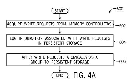
(57) Abstract: A technique includes acquiring a plurality of write requests from at least one memory controller and logging information associated with the plurality of write requests in persistent storage. The technique includes applying the plurality of write requests atomically as a group to persistent storage.
