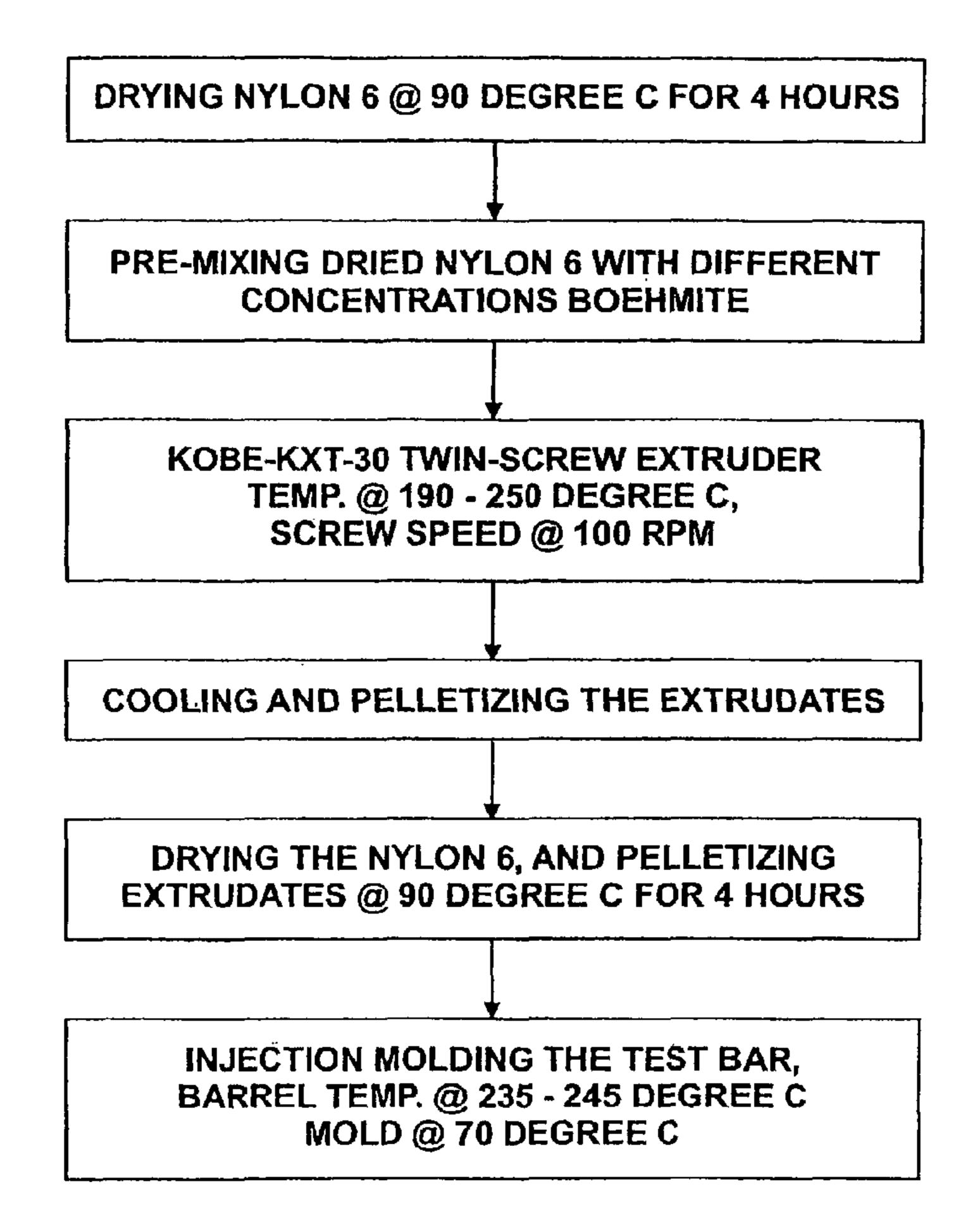
(57) Abstract: A flame retardant polymer composite is disclosed. The composite includes a polymer base material and a flame retardant filler provided in the polymer base material, the flame retardant filler containing seeded boehmite particulate material having an aspect ratio of not less than 3:1.
