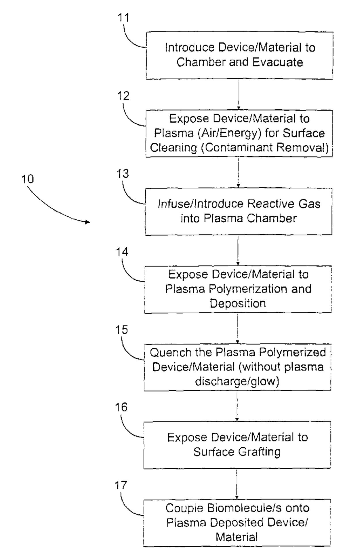
(57) Abstract: A method of modifying surfaces of a device, for example, a medical device, is disclosed. The method includes modifying a surface of a device by providing a device, exposing the device to a reactive gas and plasma energy to create a plasma deposited surface on the device, and quenching the device with the reactive gas. The device exhibits changes in its surface properties thereby making it more desirable for an intended use.
