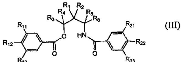
wherein R<sub>1</sub>-R<sub>6</sub>, R<sub>11</sub>-R<sub>13</sub>, and R<sub>21</sub>-R<sub>23</sub> are the same or different. Each of R<sub>1</sub>-R<sub>6</sub>, R<sub>11</sub>-R<sub>13</sub>, and R<sub>21</sub>-R<sub>23</sub> is selected from hydrogen, a halogen, and a substituted/unsubstituted hydrocarbyl group having 1-20 atoms.
