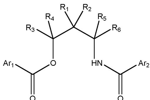
25 wherein  $R_1$ - $R_6$  are the same or different, each of  $R_1$ - $R_6$  is selected from the group consisting of hydrogen, a halogen, and a hydrocarbyl group having 1-20 carbon atoms; and
