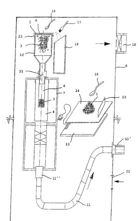
(57) Abstract: A method of cleaning pollen from mechanical impurities, spore and micro-organisms is based on the fact that dirty pollen (1) is sucked to air flow via an insulant sieve (2). Clean pollen (3) falls into a filter (6), dirt (5) sticks on the sieve (2). The pollen cleaning device consists of a sucking unit (7) with a filter (6), before which at least one sieve (2) with a throttle flap (8) is located.
