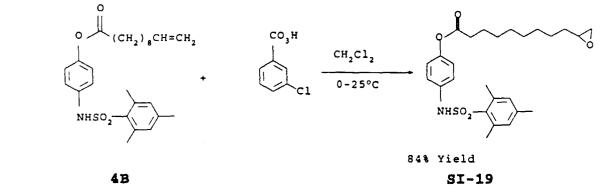
**[0082]** A 500mL flask equipped with a magnetic stirring bar and a pressure equalized addition funnel was charged with 4B (24.50g, 53.53 mmol),  $CH_2CI_2$  (150 mL). This solution was placed in a room temperature water bath. A pressure equalized addition funnel was charged with a solution of m-perbenzoic acid (80%, tech. grade; 17.30g, 80.30 mmol)
