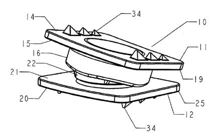
(57) Abstract: A constrained spinal implant is inserted between adjacent vertebrae to function as an disk prosthesis. The prosthesis has two plates fastened to adjacent vertebrae facing each other. The facing sides of the plates each have a depending skirt formed as concentric arcs of about 90 degrees. The skirts are either bowed or tapered in the axial direction. Depressions are centrally located between the arcs of the plates and a ball is universally movable in the depressions.
