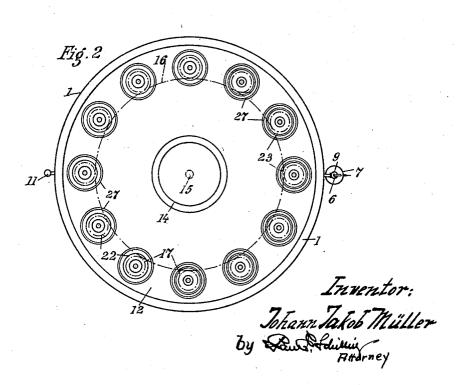
MACHINE FOR DYEING, BLEACHING, AND THE LIKE OF LOOSE YARNS OR BOBBINS
