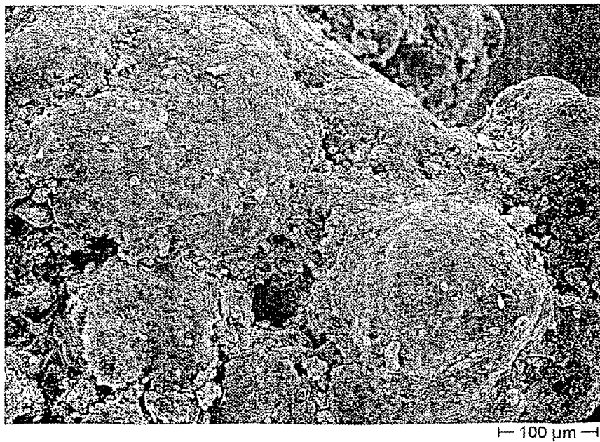
Figure 12B: Surface of Nal-10-Sure granulates at 200x magnification. The voltage was 10 kV. The bar length corresponds to 100 \mu m.
