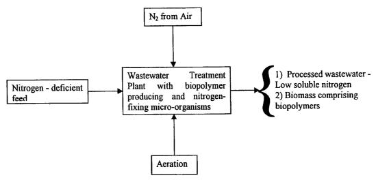
(57) Abstract: A process for producing biopolymers comprises passing nitrogen deficient wastewater through a treatment system comprising micro-organisms which grow aerobically in nitrogen deficient wastewater, and controlling the environment in the treatment system by maintaining a sufficiently stable dissolved oxygen level to thereby encourage the growth and/or activity of micro-organisms which produce the biopolymers, and recovering the biomass produced and the biopolymers.
