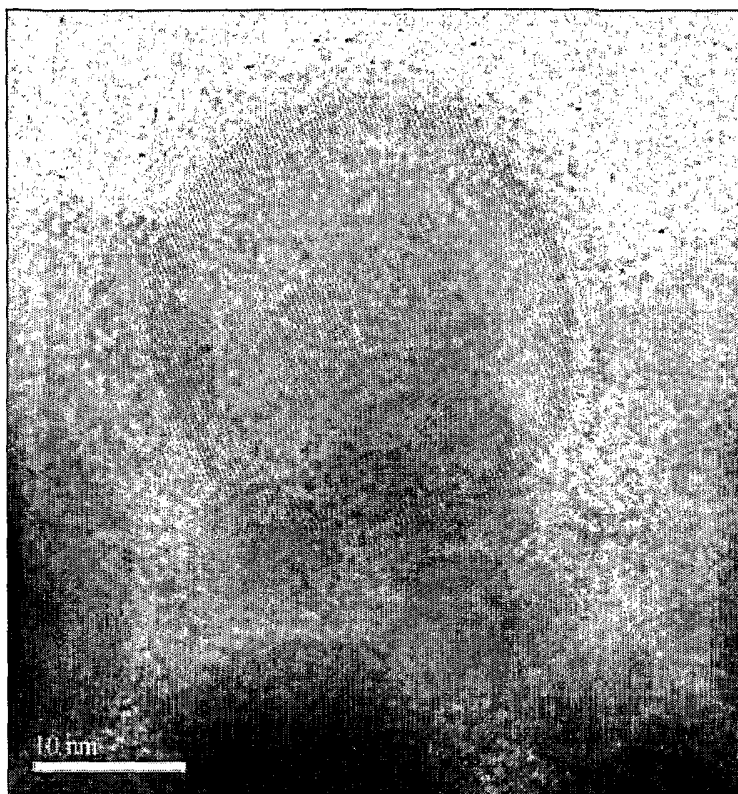
Figure 10- Core-Shell Nanoparticles. TEM studies appear to show that the nanoparticles that compose the agglomerates have a 'core-shell' structure. The outer layer (top particle, about 3nm thick) appears to amorphous, and the inner core is clearly crystalline ceria.
