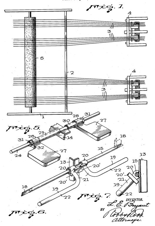
PORTABLE LOOM CREEL AND ADJUSTING MEANS THEREFOR
