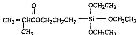
This kind of coupling agent reacts with the colloidal particles such that the  $\text{SiO}_x$  moiety bonds to the particles, while the carbon-carbon double bond remains available for copolymerization with the curable binder component to the extent the curable binder component includes radiation curable materials. Typically, about 10 parts by weight of the surface treatment agent is used per 100 parts by weight of colloidal particles.
