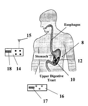
(57) Abstract: A medical device (8) includes a device body (12) for insertion into an organ of a patient and one or more arms (10), which are attached to the device body and are arranged to extend outward from the device body within the organ so as to contact respective points-of-contact on an inner surface of the organ, and to apply a repetitive motion at one or more of the points-of-contact.
